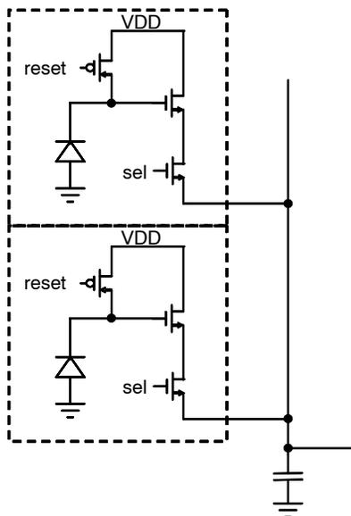
Figure 8. Active Pixel Cell Architecture
