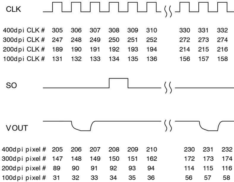
**Figure 7. Timing of SI/SO Clock for 400/300/200/100 dpi Modes**
