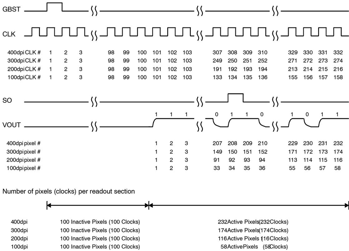
**Figure 4. Overall Timing Diagram for 400/300/200/100dpi Modes**
