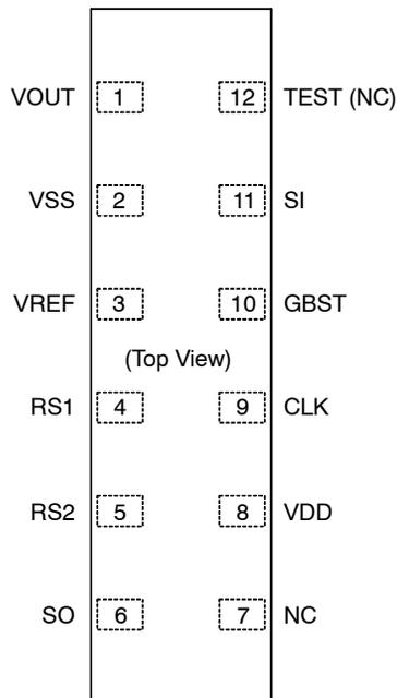
Figure 2. Pinout Configuration
